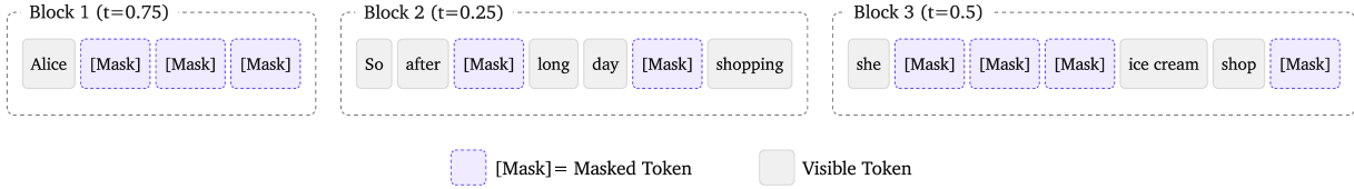
Figure 18. Per-block masking schedule. Each block samples an independent noise level t_b \sim \mathcal{U}(0, 1) , so blocks in the same sequence are denoised to different degrees within a single training step.
